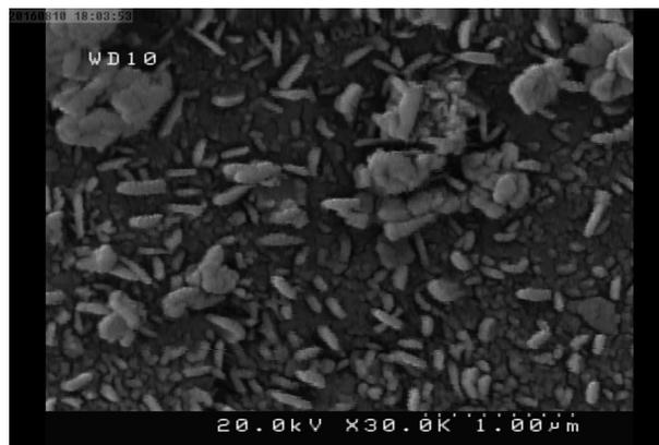
Figure 1. Scanning Electron Microscopic Image of Nano-MgO Dry Powder
